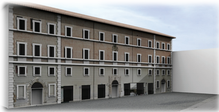
Figure 13. 3D model of Palazzo della Famiglia in Piazza Borghese. The elevation is textured by projecting the equi-rectangular image from the Google panorama.
