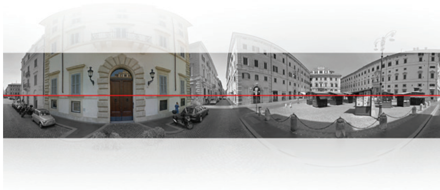
Figure 15. Panoramas with a lot of sky represented, determine errors in the upper and lower part of the image, because of few homologous points to connect the frames.
