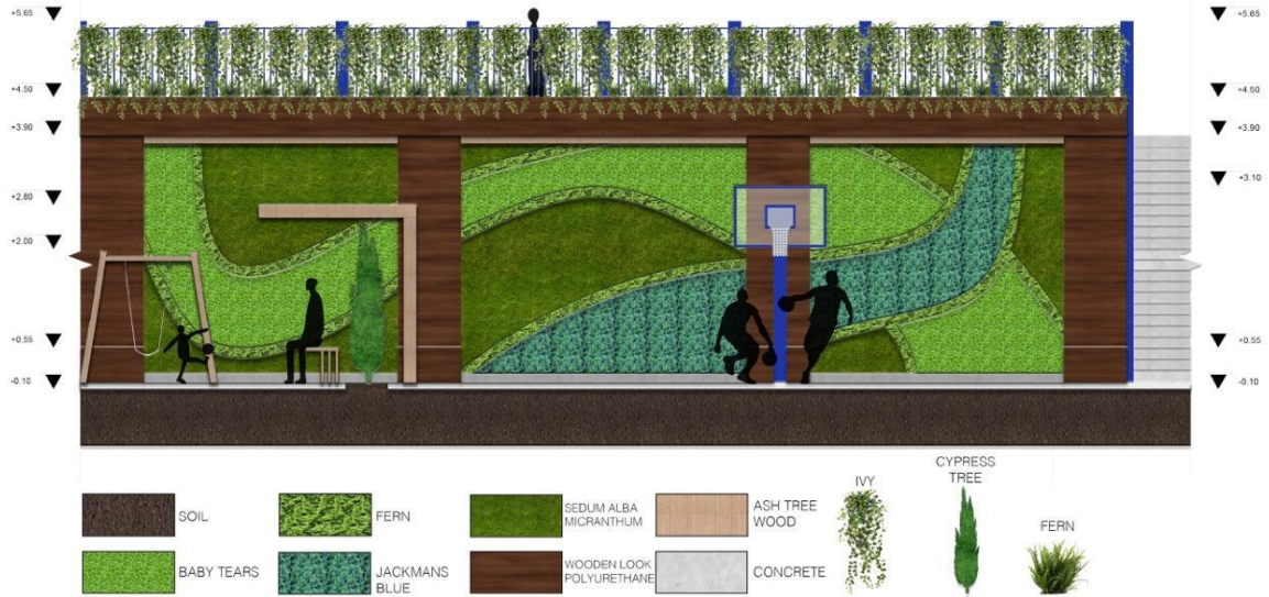
Fig. 10. Vertical garden area partial section drawing 1/50 scale
